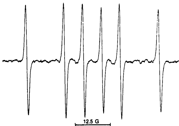
FIGURE 3 EPR spectrum of DMPO-Ar spin adduct from system containing amine 13 (0.1 M), DMPO (10 mM) and iAmONO (3.5 mM) in deaerated benzene. HF coupling constants are given in Table 3.
